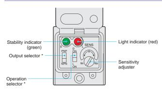
$<sup>^{\</sup>star}$  Use the output selector to select the type of output transistor, NPN or PNP.
